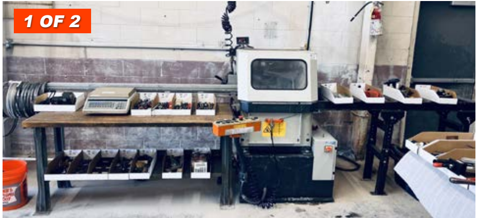
Elumatec MGS 500SP Semi-Automatic Circular Mitre Saw
